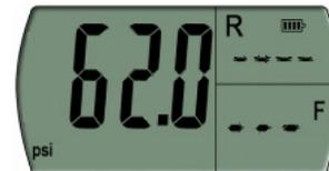
9. If needed, press "R" button to select the type of refrigerant you will be working with. Press "R" button until desired type of refrigerant is shown. Gauge will acknowledge selection by blinking chosen refrigerant number for 3 seconds after selection is made.
