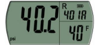
8. The display will show last stored features (pressure and temperature units, refrigerant type) and current pressure/corresponding temperature reading:
