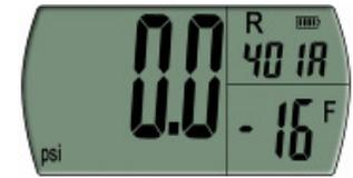
5. The gauge should be turned off again before the application of pressure. Press ON/OFF button and hold for 2 seconds, gauge will go off.
