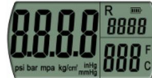
7. Press "ON/OFF" button, all digits light up for 2 seconds. (The battery capacity always shows on display).
