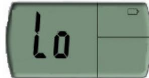
When Battery capacity is between 25% and 50%, display shows:
