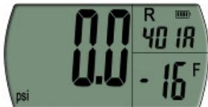
3. LCD will show 0.0 pressure and previous Refrigerant Type and last recorded temperature.
